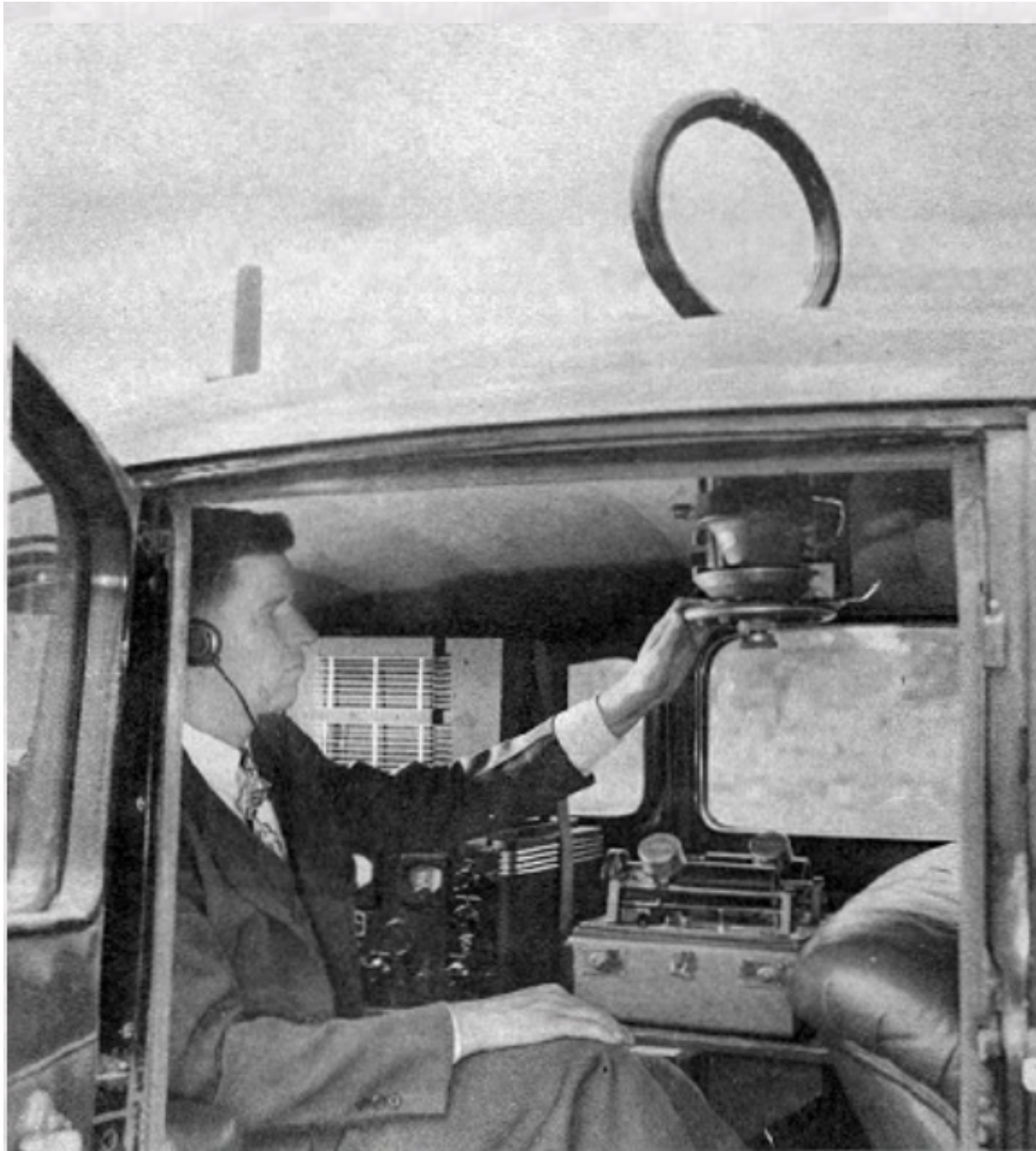
Internal view of RID prowler car used to intercept signals and locate sources of interference. The loop did not show while the car was cruising but only when taking a bearing. Equipment included an SX-28, dictaphone recorder and other receivers covering 75 Kc to 300 Mc.
