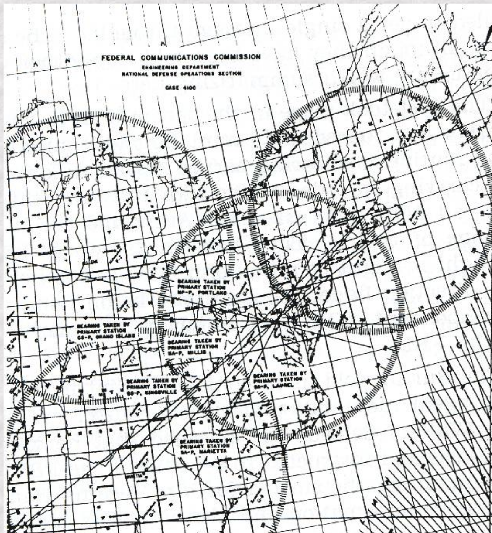
Plot of bearings taken by RID primary monitoring stations to determine the location of a clandestine transmitter in Washington, DC area on December 9, 1941. The first alert was sounded by an aperiodic receiver in a mobile unit cruising DC that was immediately followed by an alert from the primary monitoring station in Portland, Oregon.
