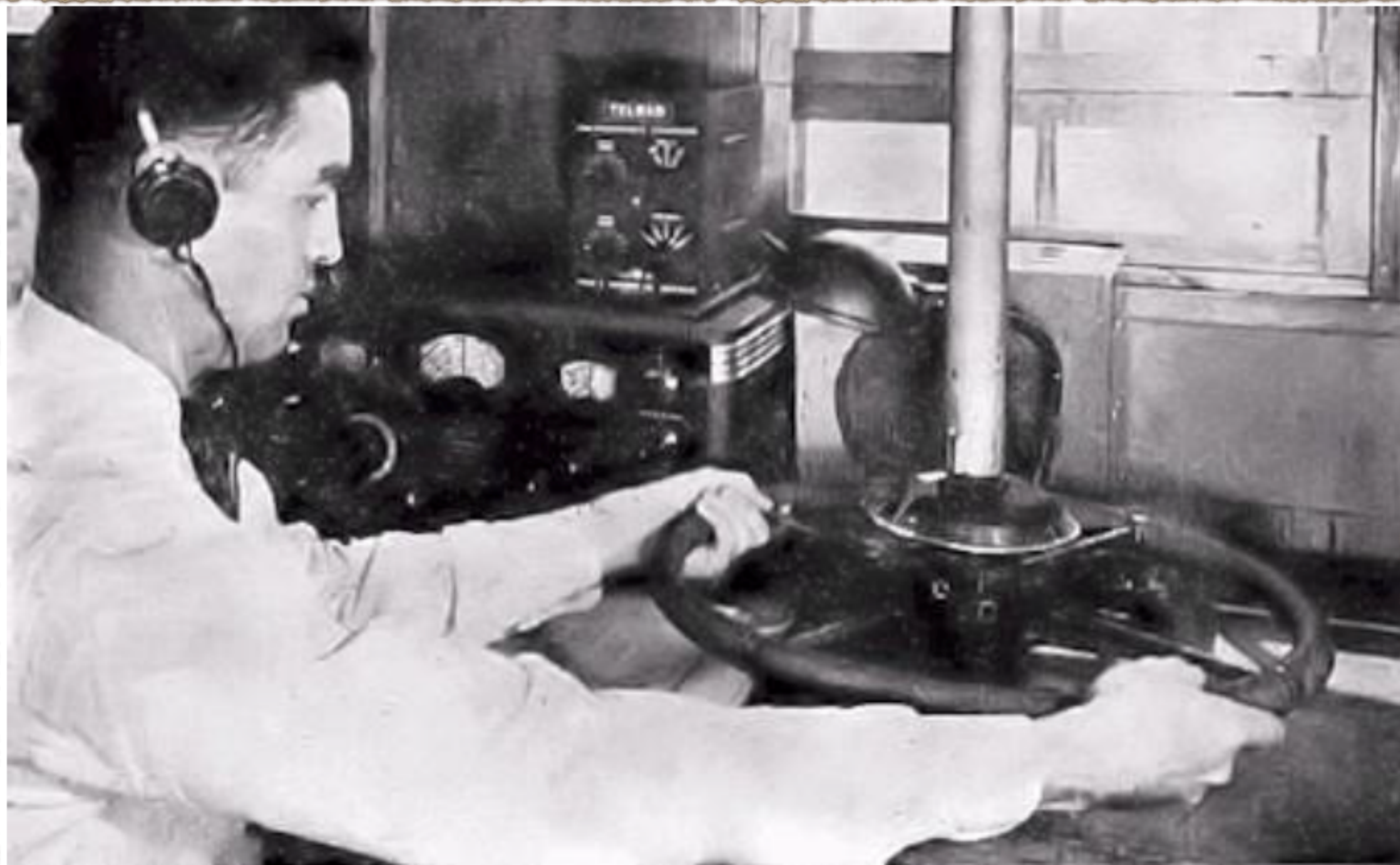
Figure 30: Assistant Supervisor K.W. Miller, W5AOC, taking a bearing with an Adcock direction finder. The antenna was rotated to obtain a null in signal strength. At this point the antenna is broadside to the direction of arrival of the signal.
