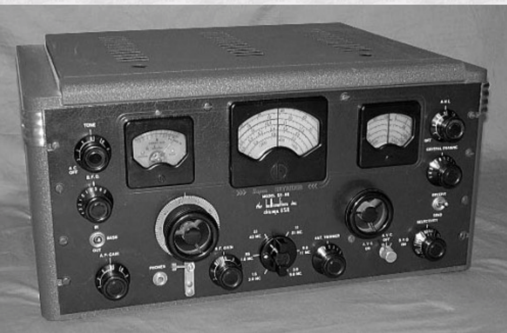
Hallicrafters SX-28 was the workhorse receiver used by the FCC/RID monitoring stations and mobile units.
