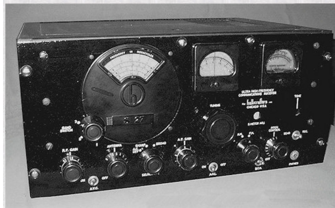
Hallicrafters S-27 receivers were also used by the FCC/RID monitoring stations and mobile units.
